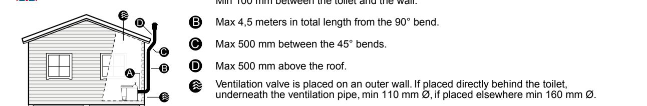
*NOTE! Only Ø110 mm vent.pipes made of plastic and 1pcs 90 ° bend may be used in the installation.*
