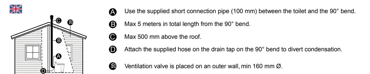
**NOTE!** Only Ø110 mm vent.pipes made of plastic and 1pcs 90 ° bend may be used in the installation. When installing a 90 ° bend tube directly behind the toilet, 30 cm space is required for installation behind the toilet.
